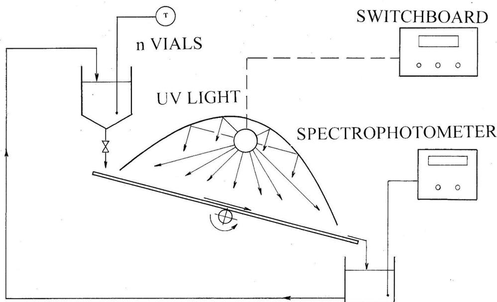
INCLINED FLOW-THROUGH REACTOR
