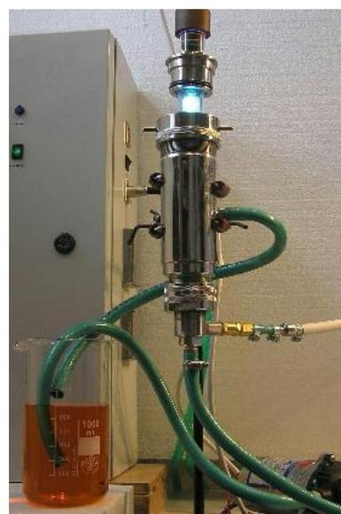
Fig. 1: Flow-through annular reactor
