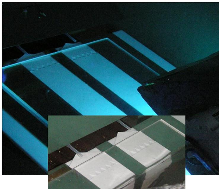
Fig. 4 Inclined flow-through reactor - individually flooded strips of filter cloth under UV illumination, entrance edge and flow distributors (in detail)
