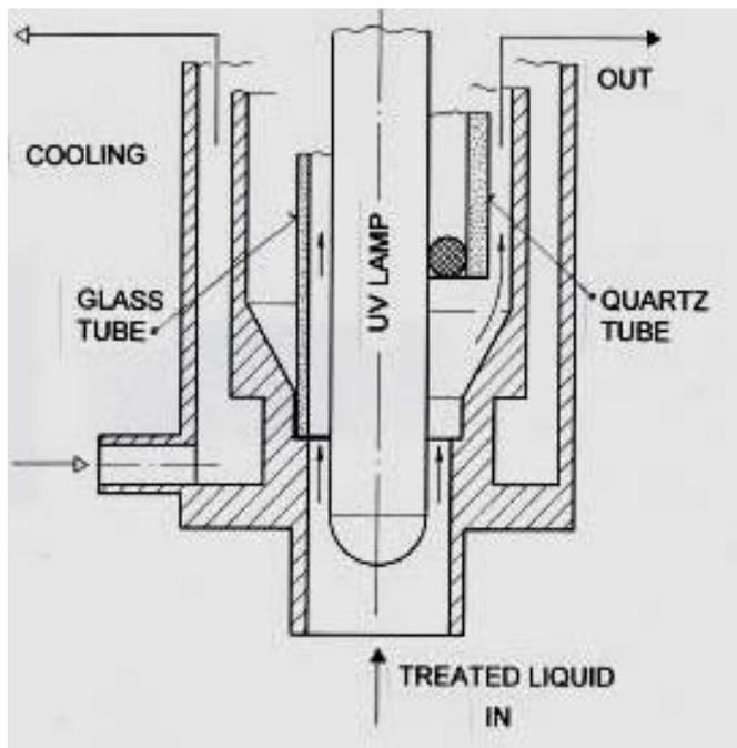
Fig. 2: Cross-section of the flow-through annular reactor
