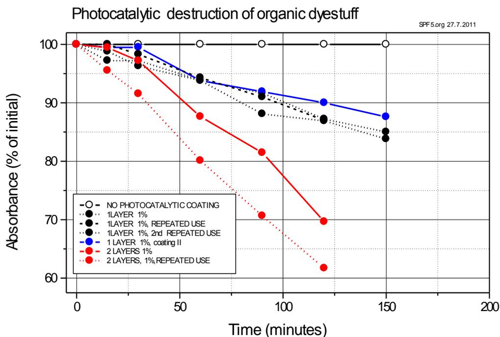
Fig. 5. Evaluation of photocatalytic efficiency of several coatings on non-woven glass textile
